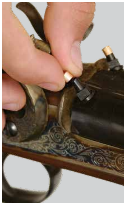
The final step before firing is capping the nipple.
